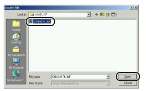
13 Make sure that the correct path is displayed in the [Copy manufacturer's files from] field, then click [OK].
